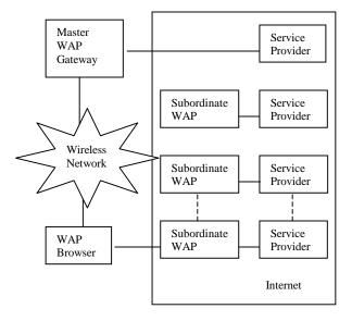
Fig 4-4 Transport Layer in an end-to-end Security Architecture
