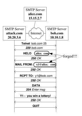
Figure 7: Spamming - sender address spoofing
