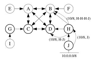
Figure 8: Changing traffic flow by AS\_PATH falsification
