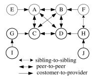
Figure 3: A simple AS topology with different types of AS relationships.
