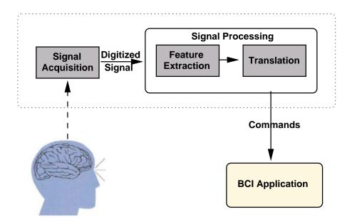
Figure 2: Basic design of a BCI system [55].
