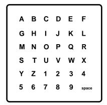
Figure 3: Illustration of a screen intended to randomly highlight letters (from the spelling device in [4]). The technology exists such that this approach could be used for a pass-thought system.
