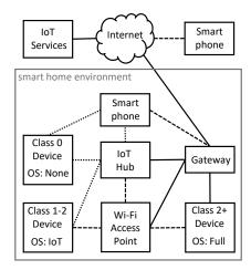
Fig. 2. Generic architecture of smart home IoT deployment. Solid lines denote wired connections, thick dashed lines represent Wi-Fi, thin dashed lines represent low-power wireless, e.g., Zigbee, Bluetooth Low-Energy. "IoT" OSs are specifically for IoT devices (Section III-A). "Full" OSs are, e.g., Linux.
