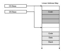
Figure 7. Splitting the flat memory model to allow a tamper resistance attack
