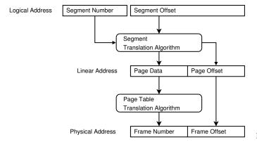
Fig. 4. Translation from virtual to physical addresses on the x86
