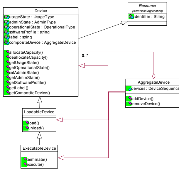
Figure 8. Class diagram for devices.
