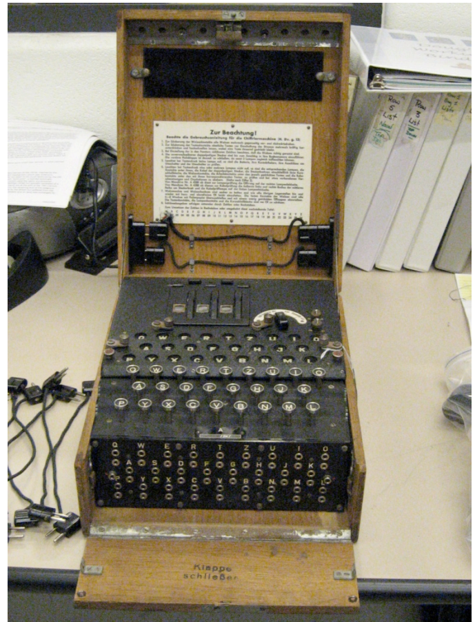
The Type A Enigma owned by the Canadian War Museum (Ottawa). Note that this version has only three rotors. (Photo by the author)
