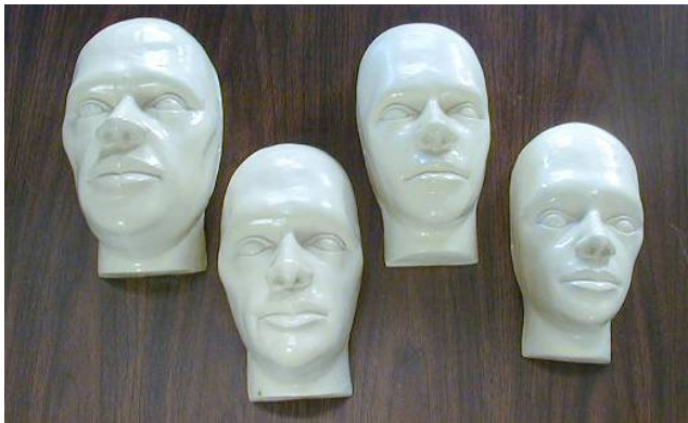
Figure 1 Sculpted head forms for respirator design.
