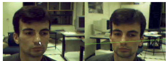
Fig. 7. Examining the quality of stereo calibration. The features to be tracked must lie on the epipolar lines.
