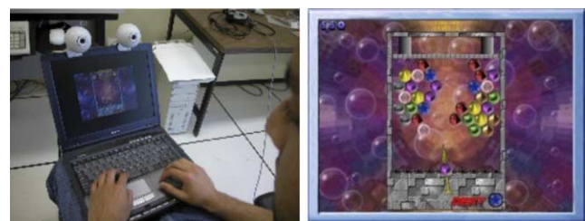
Fig. 13. Setup for stereotracking. A user plays an aim-n-shoot game aiming with his nose.
