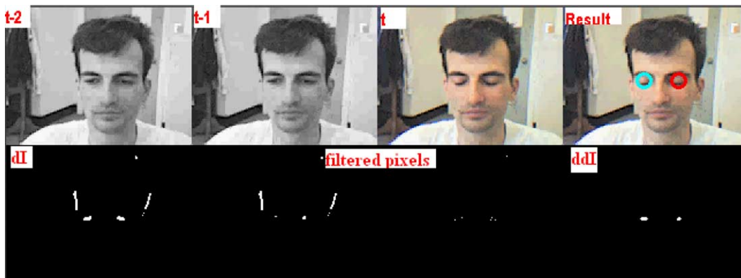
Fig. 10. Detection of eye blinks using the first order (bottom left image) and the second order change (bottom right image) detection. The pixels change due to head motion are shown at the bottom center images.
