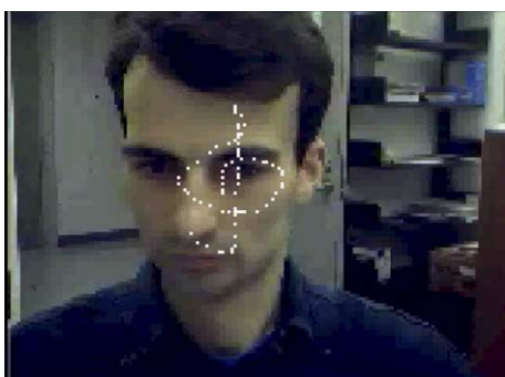
Fig. 4. Drawing the G-clef sign with head motion. Shoulders are held still.
