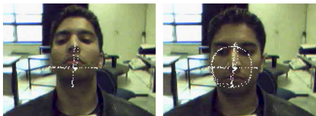
Fig. 3. Tracking ‘Yes’, ‘No’ and circular motion. Shoulders are held still.
