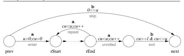
Figure 5.2: The internal representation of repeating symbols Internally, qcap unrolls the last repetition of a region with a cardinality greater than one, resulting in the transition, unrolled being added to the finite automata.
