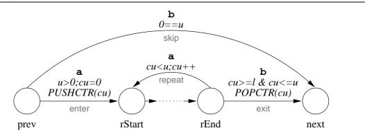
Figure 4.7: An automata modified to handle a dynamic cardinality, and maintain the counter stack
