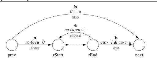
Figure 5.1: An automata modified to handle a minimum and maximum dynamic cardinality
