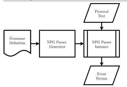
Figure 1.1: Flowchart illustrating the position of the Network Protocol Grammar in the network monitoring tool chain.
