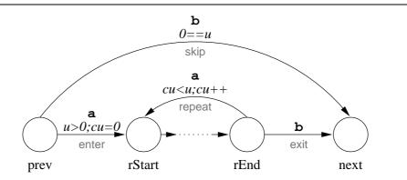
Figure 4.3: An automata modified to handle a maximum dynamic cardinality The structure of an automata that handles dynamic maximum cardinality.
