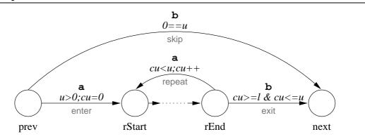
Figure 4.4: An automata modified to handle a minimum and maximum dynamic cardinality
