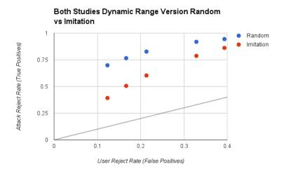
Figure 6.8: ROC curve comparing version 2 for two different attacker datasets
