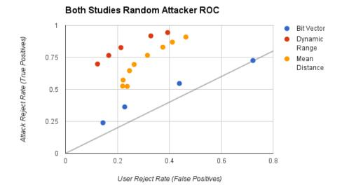
Figure 6.6: ROC curve comparing three versions of the algorithm for random data
