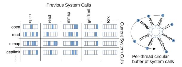
Figure 2.5: Building a training profile from a system call sequence: open, read, mmap, mmap, open, getrlimit, mmap, read, read, write, fork, close and window size 8.
