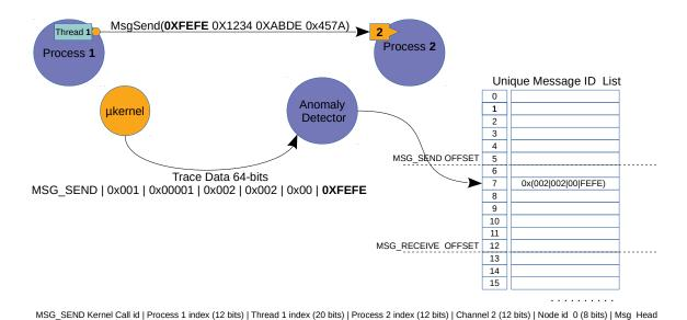
Figure 4.3: How a message is traced and stored in tH's data structures.
