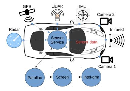
Figure 5.1: The various sensors and processes used to record and replay sensor data.
