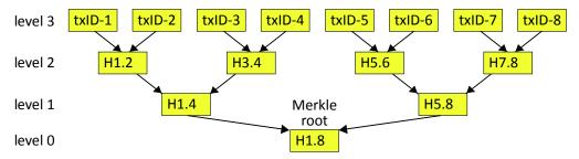
Figure 13.5: *Merkle tree* of transaction hashes (hash tree, *authentication tree*). Each node holds a 32-byte hash value. The leaf nodes are the hashes of respective transactions.
