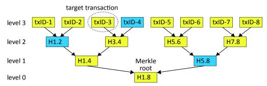
Figure 13.10: Merkle path authentication. Off-path values for txID-3 are shaded (blue). A block having N transactions has an *authentication path* involving only  $lg_2(N)$  values.
