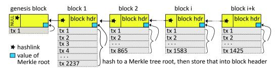
Figure 13.6: The full blockchain. A block header's hashlink (Fig. 13.1) holds the hash of the block header pointed to, allowing verification of the integrity of the pointed-to block. The genesis block (hard-coded into nodes) serves to validate the final integrity check.
